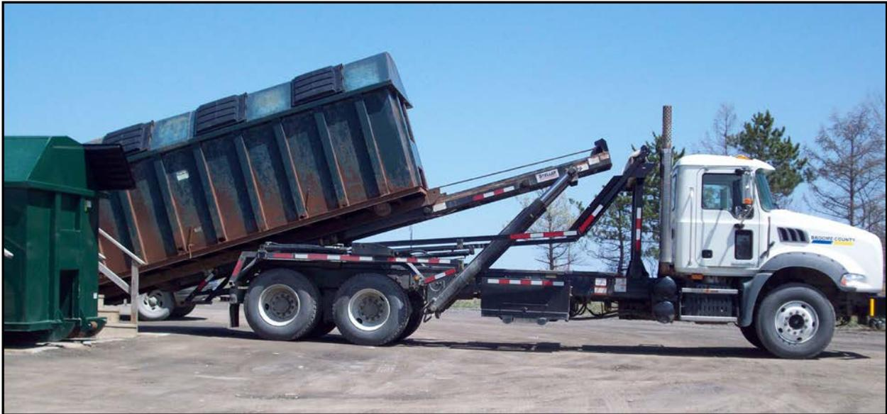
Photo 4: Pulling Recycling Roll-off
